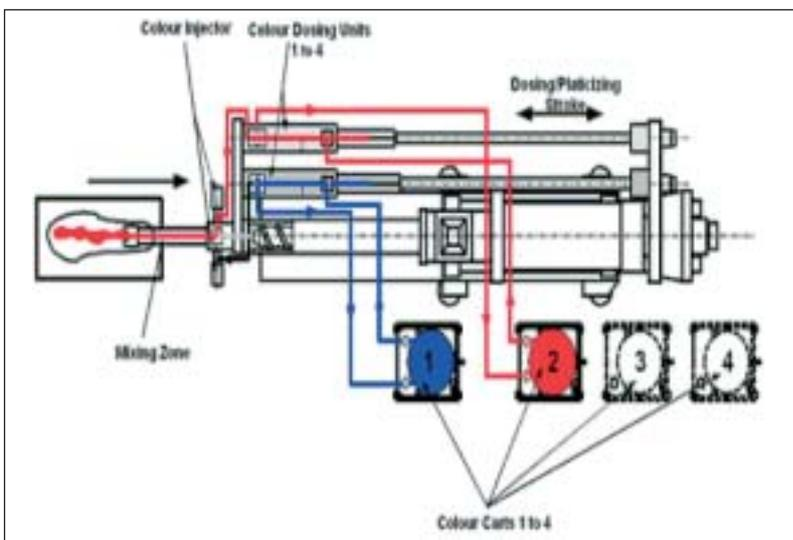
Fig. 9: Principle of the Desma colour addition method
