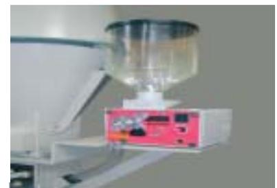
Fig. 5: Addition of dry colorant according to the masterbatch method
