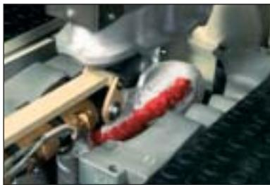
Fig. 8: Pouring process according to the DESflow principle
