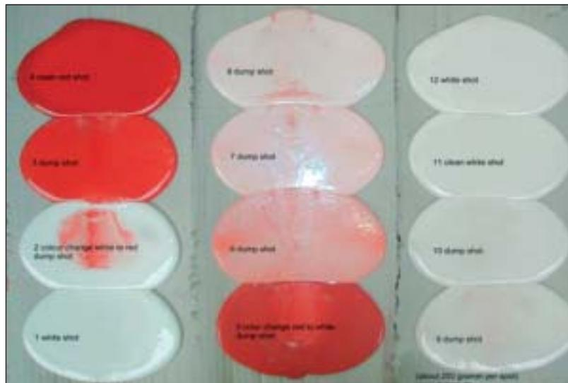
Fig. 1: Example of a colour change-over with Desma technology
