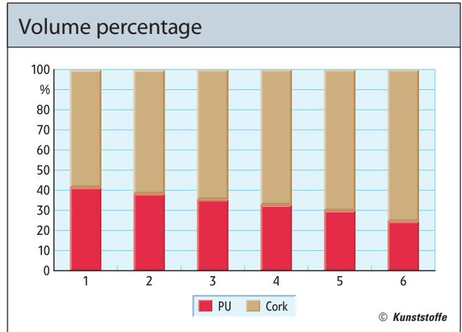
Fig. 5. The limiting range (No. 6) is achieved at a mixing ratio of 75 vol.-% cork and 25 vol.-% PU
