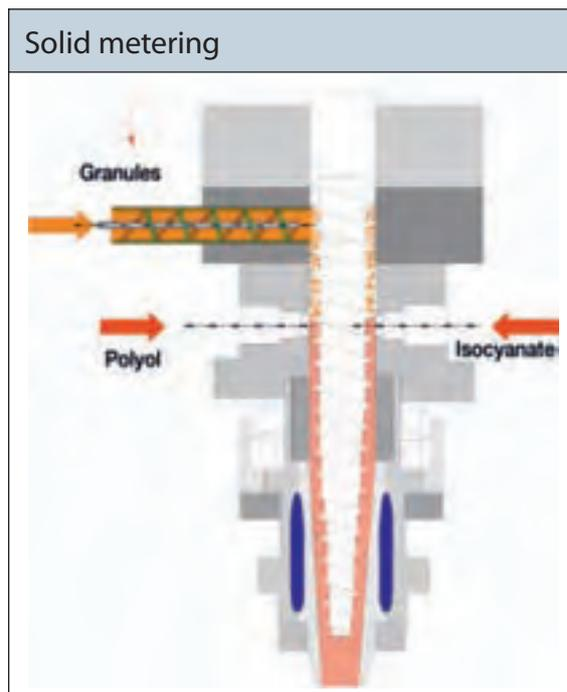
**Fig. 3. Mixing head with integrated solid metering**
