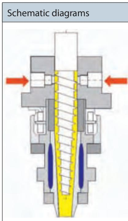
**Fig. 1. Construction of the mixing chamber with high-speed screw and valve plane**
