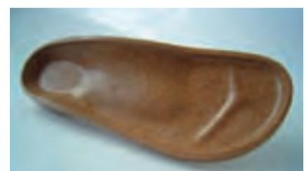
Fig. 8. Example of a cork/PU shoe sole with a proportion of 15 wt.-% cork
