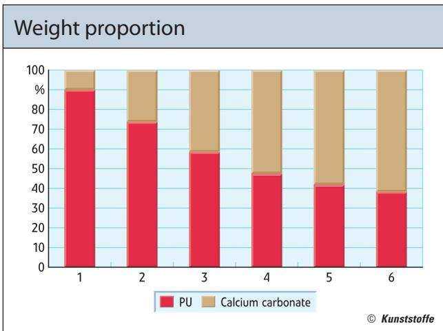
Fig. 6. The limiting range (No. 6) is achieved at a mixing ratio of 61 wt.-% calcium carbonate and 39 wt.-% PU
