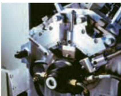
**Fig. 2. The mixing head with three component valves and positive synchronisation permits high quality without premature advance of one component**
