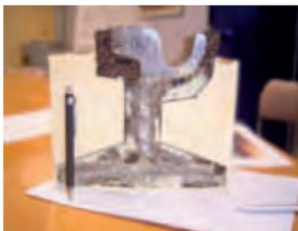
**Fig. 9. The rail bed cast with cork/PU reduces the rolling vibrations of the tram**
